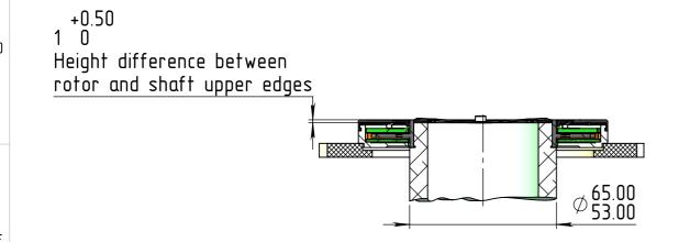
Shaft end with shoulder mounting — example mounting by special spring ring
